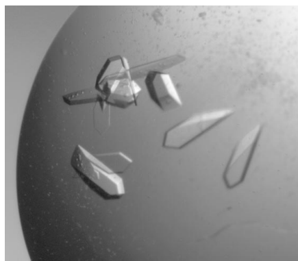
Figure 1 Photomicrograph of crystals of AVP. Prism-shaped crystals of AVP obtained by microseeding were used for X-ray diffraction. The typical crystal dimensions were 0.05 × 0.15 × 0.50 mm.
